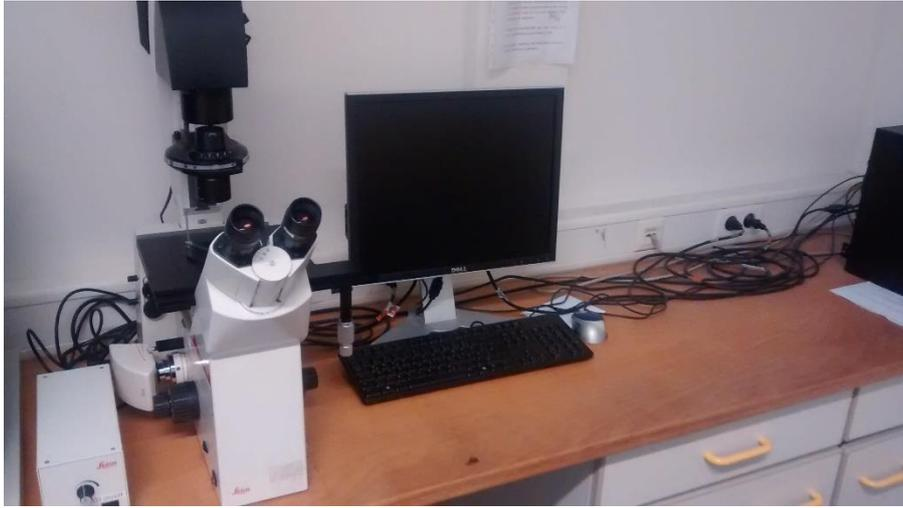
*Figure 15: Leica optical microscope*
