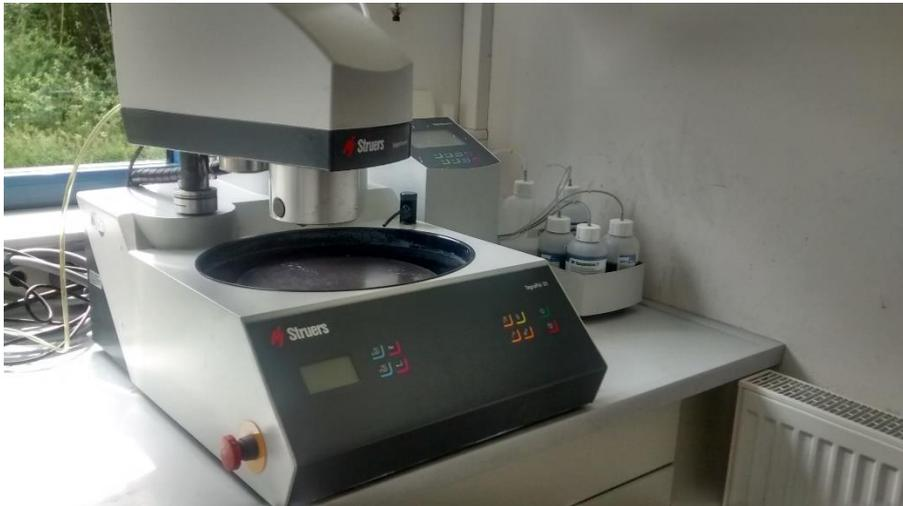
*Figure 16: Grinding and polishing machine*
