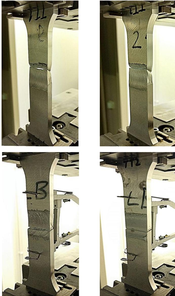
*Figure 30: Fracture position of Tensile test: Al side for E6 and E7 and joint line for E8 and E9*
